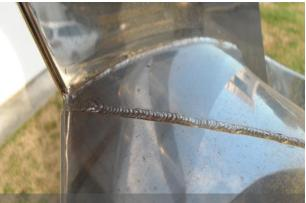
External corner welds ground and polished to mirror. Internal fillets and butt welds left as laid, polished to mirror.
