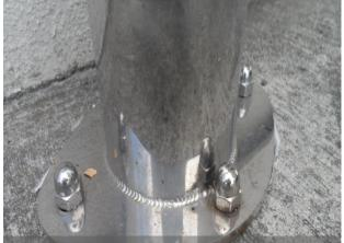
Fillet weld. Left as laid, polished to BA. Note "tea staining" after 1 year in service.
