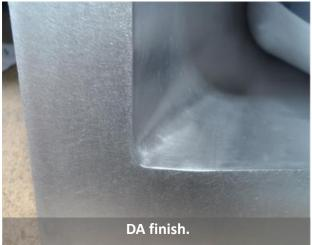
Internal Fillet weld ground and polished.
